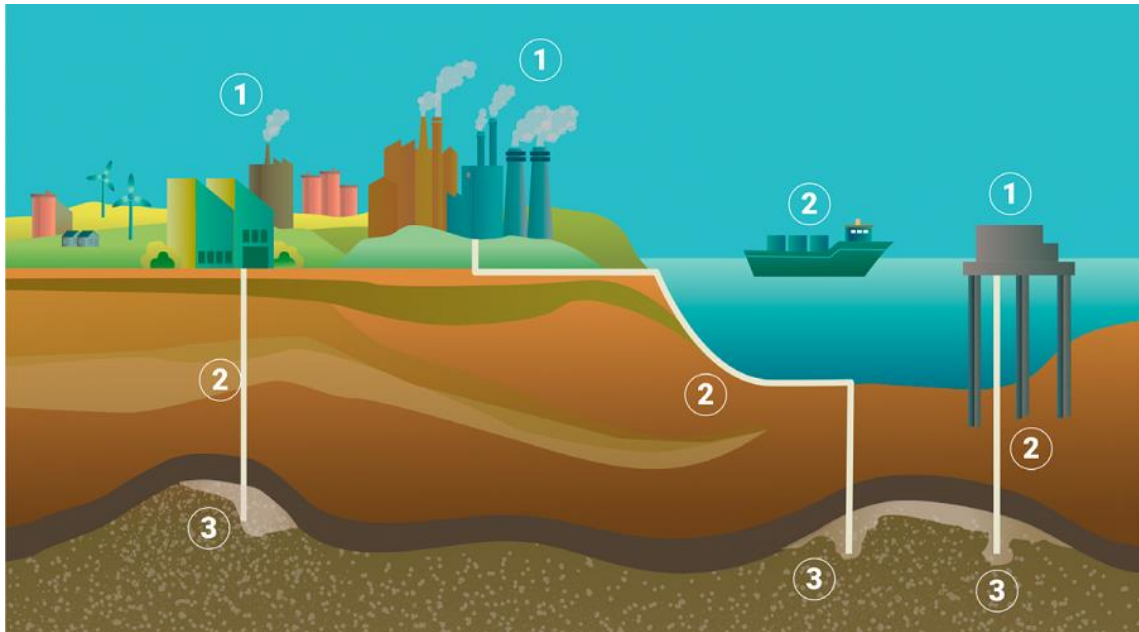
Figure 2.1 Graphical representation of the CCS value chain: interaction between capture, transport and storage.
